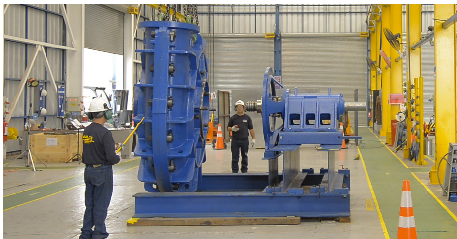
Above: A new innovative quick change procedure has been developed for faster removal of the larger mill circuit pump wet ends.
