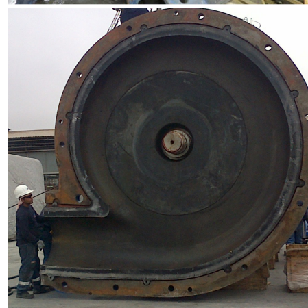
Top: Reinstalling Warman® MCR® 550 pump suction cover after impeller and throatbush inspection.
